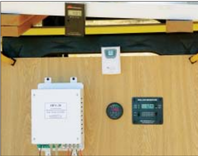
To keep tabs on every aspect of the testing procedure, all requisite controls and monitors were mounted nearby, including a regulator, amp-hour meter, the HPV30 controller, an outdoor thermometer and an insolation meter.
